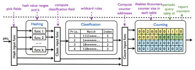
Figure 2: OpenSketch switch data plane
