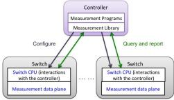
Figure 1: Software defined traffic measurement
